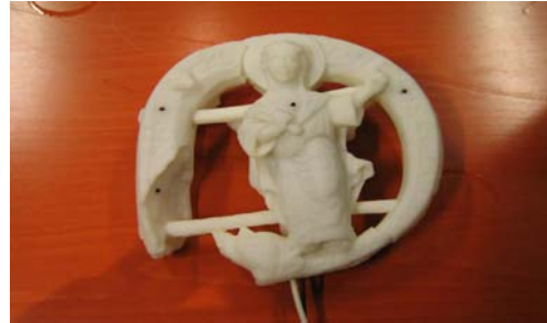
Fig. 5: Kromstaf replica with touch and orientation sensors
